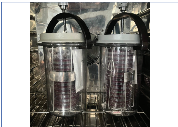
[Table/Fig-3]: Anaerobic jar with gas-pack system for oxygen-free incubation of blood agar plates for anaerobic culture.
